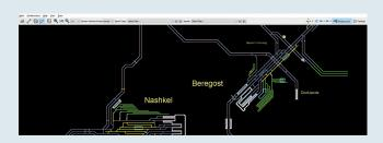
The **GEOGRAPHY EDITOR** is a "digital copy" of the railway network and infrastructure. The microscopic modeling of the network allows high-precision timetable management. Line closures, construction sites etc. can be seen at a glance.
